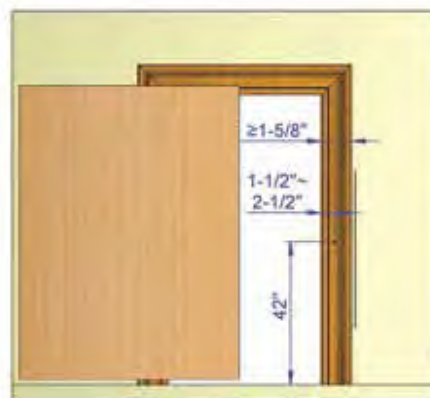
Figure 3. Proper measurement guidelines for applications with trim casing, both wide and narrow.
