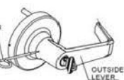
B: Turn key 90 degrees, insert push pin into hole in outside lever to depress catch.
