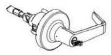
E: Insert key to check key function and make sure lock function is correct.
