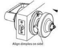
2E: Remove inside lever and install inside rose, make sure inside rose is fully snapped in.
